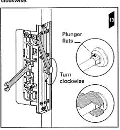
14. Continue to turn the spanner until there is no longer a gap between the spanner and the chassis.
