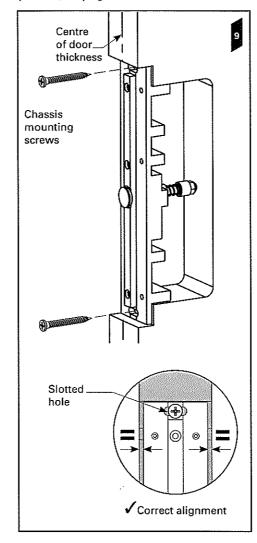
10. Fit the 6x side handle to chassis screws. Leave a 3mm gap (1/8") between the underside of the screw head and the
