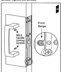
16. Use the ball end of the CL400 Allen key to fasten the 2x M3.5 screws as tight as possible. Use the other end of the Allen key to fully tighten the screws. It is important that they
