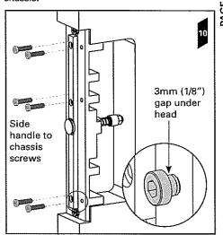
11. Fit the passage side handle (with no visible fasteners) to the chassis by sliding the front flange of the handle under the heads of the 3x side handle to chassis screws.
