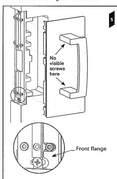
6. Fit the remaining Bi-Parting side handle to the chassis and tighten the 3x side handle to
