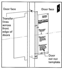
2. Mark two holes in the centre of the door thickness in the positions shown. Using these marks, drill two 2.5mm (3/32") diameter holes to a depth of 35mm (1-3/8").
